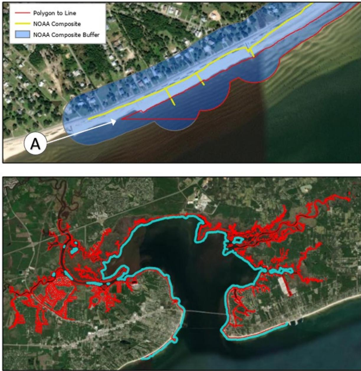
Figure 6: After converting the polygon to line, the line is split at the two points where the buffer intersects the shore (A, Top, is one example), then all lines representing the buffer over the water surface are selected and deleted (Bottom). Image Source: Esri, Maxar, GeoEye, Earthstar Geographics, CNES/Airbus DS, USDA, USGS, AeroGRID, IGN, and the GIS User Community.
