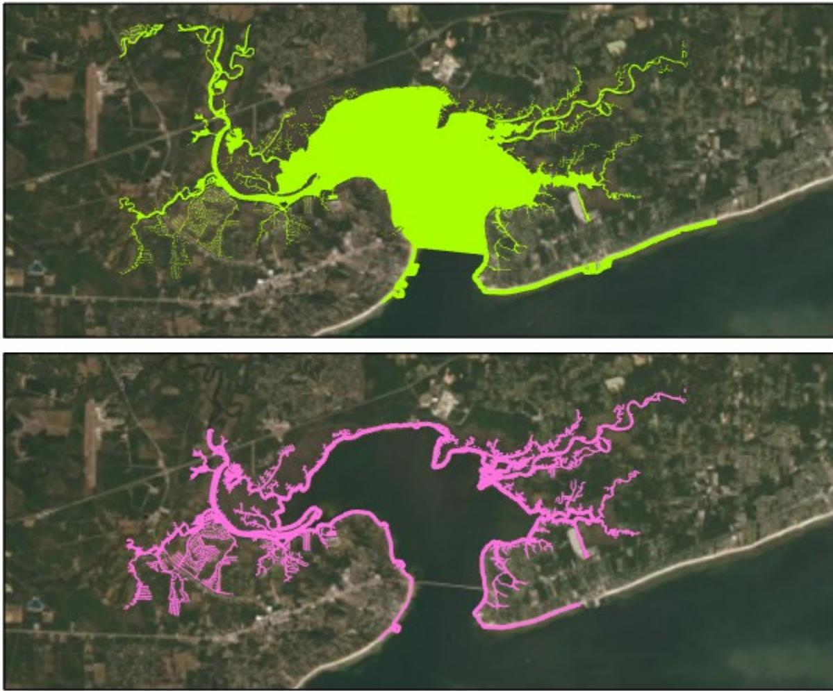
Figure 5: Polygon of below-zero elevation values derived from DEM (Top) and then clipped to 120-meter buffer of the NOAA Composite shoreline (Bottom). Image Source: Esri, Maxar, GeoEye, Earthstar Geographics, CNES/Airbus DS, USDA, USGS, AeroGRID, IGN, and the GIS User Community.
