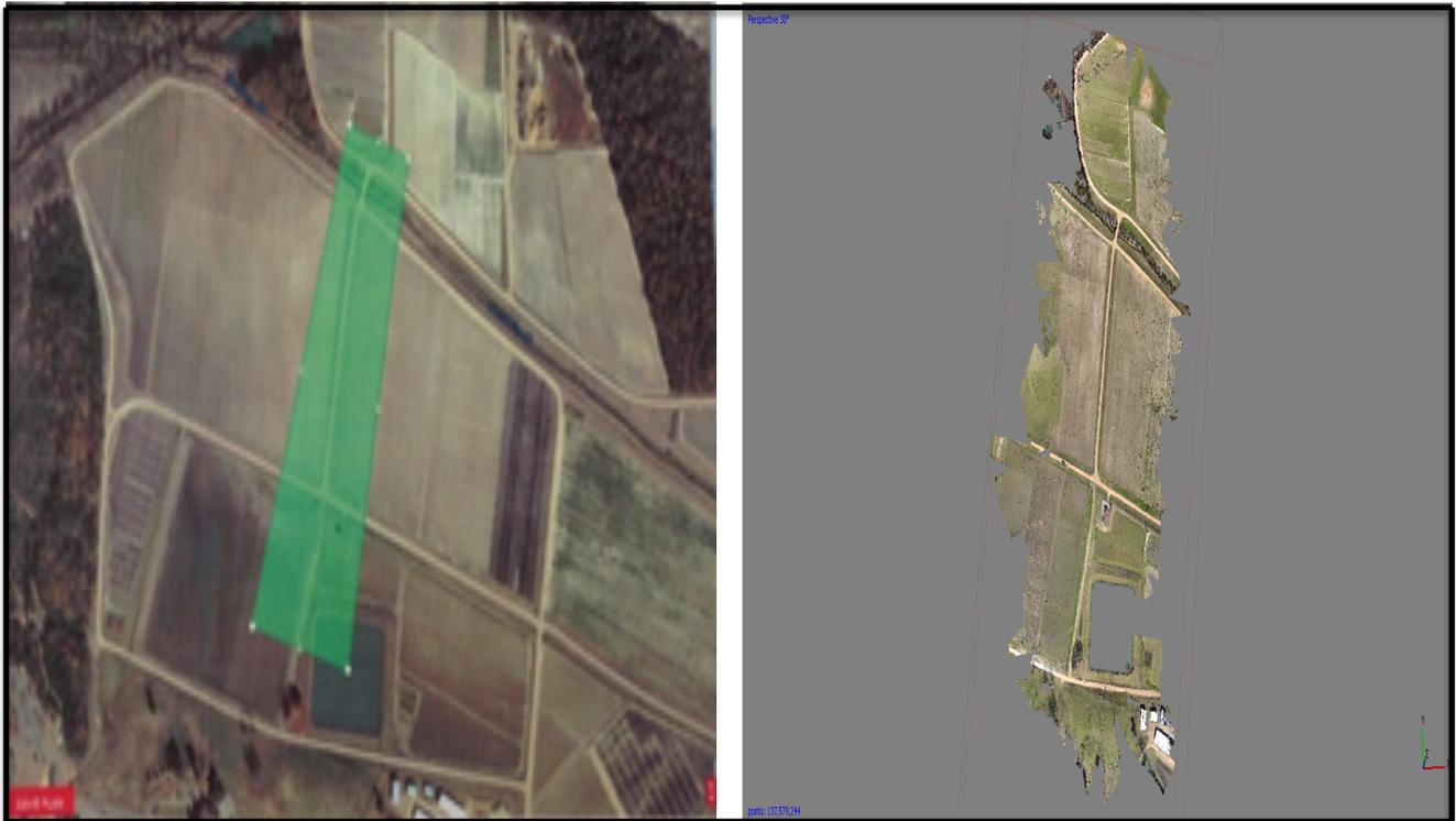
**Figure 1.** Flight plan over the R.R. Foil Plant Research Center at Mississippi State University (left) and imagery collected over the same site (right).
