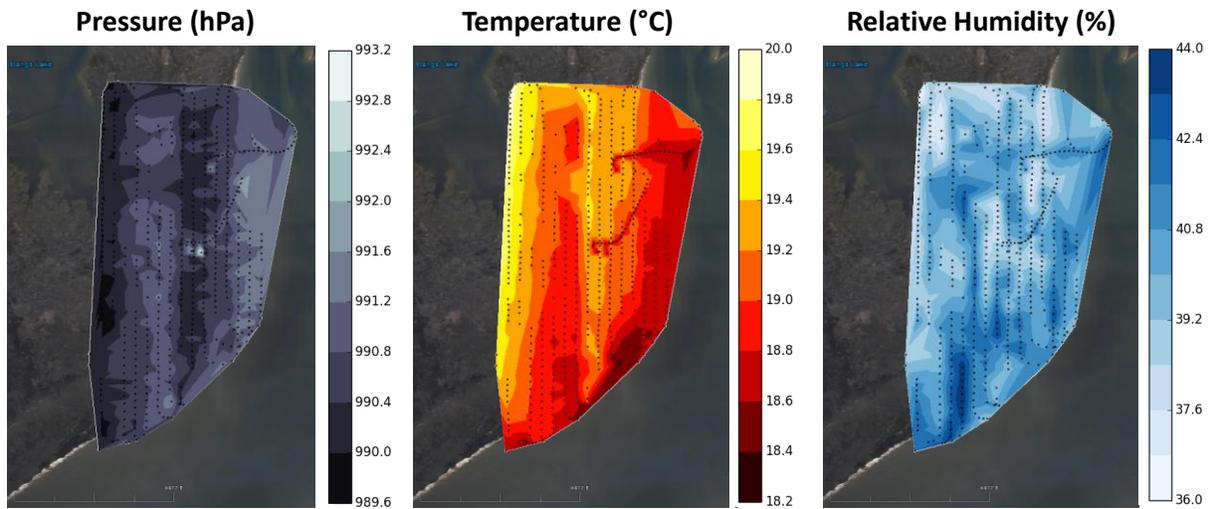
**Figure 3. UAS-measured pressure, temperature, and relative humidity at 225m AGL altitude over the November 20, 2015 test flight over Grand Bay NERR test flight. Black points represent UAS observation locations.**
