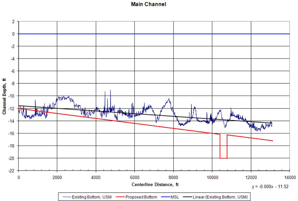
Figure 30 Sediment Trap Profile for Main Channel
