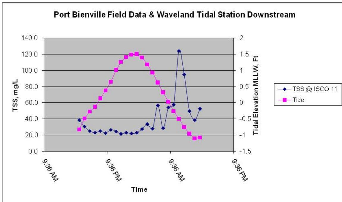
Figure 20 ISCO 11 Samples Entrance of the Port
