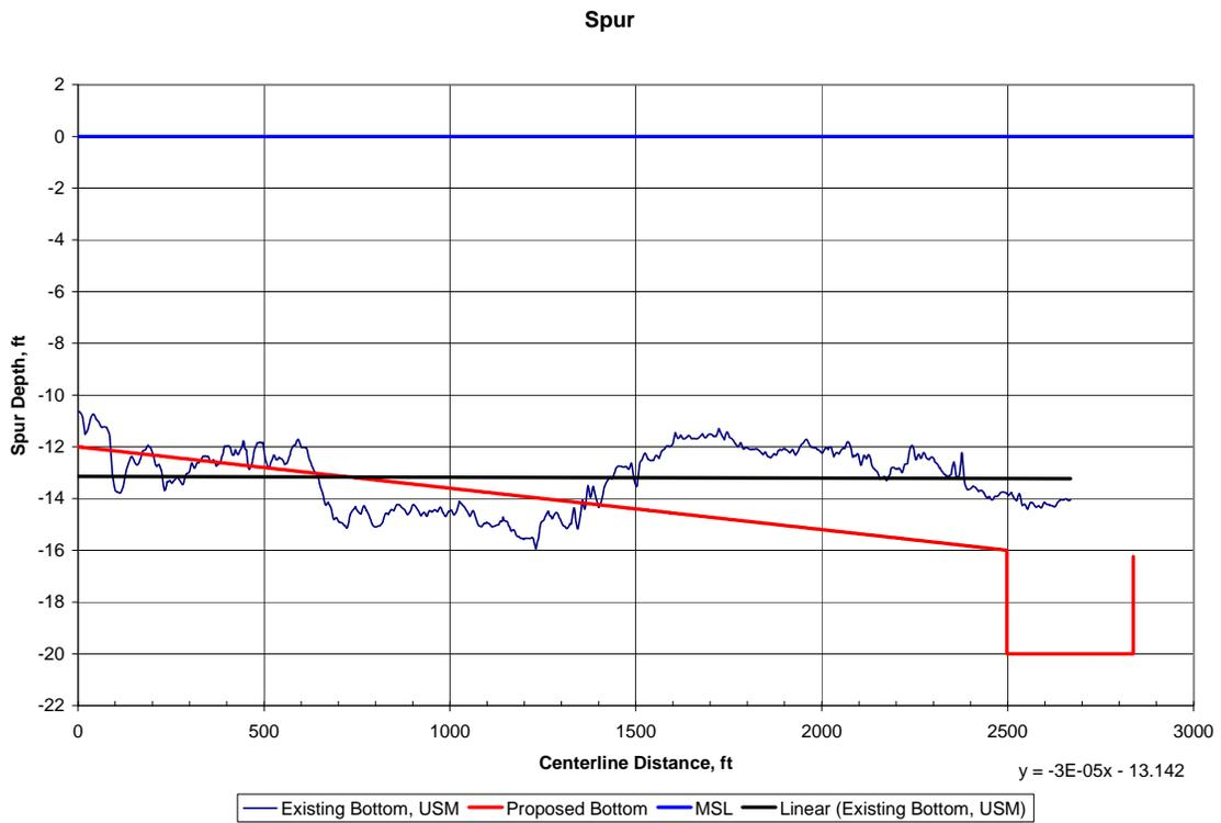
Figure 31 Sediment Trap Profile for Spur
