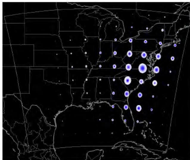
(a) Graduated uncertainty glyphs on the entire grid calculated for pressure at 1800 on 13 March.
