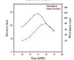
Fig. 4. ADCIRC simulation of the surge (feet) and the wind forcing (mph) for an inland point near Bay St. Louis, MS during landfall.
